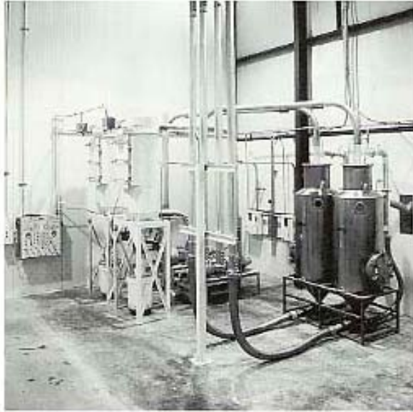
Typical installation showing a twin-pot application used in a railcar unloading system.
