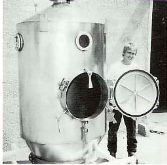
Photo illustrating large 20" access port for ease of maintenance and cleaning.
